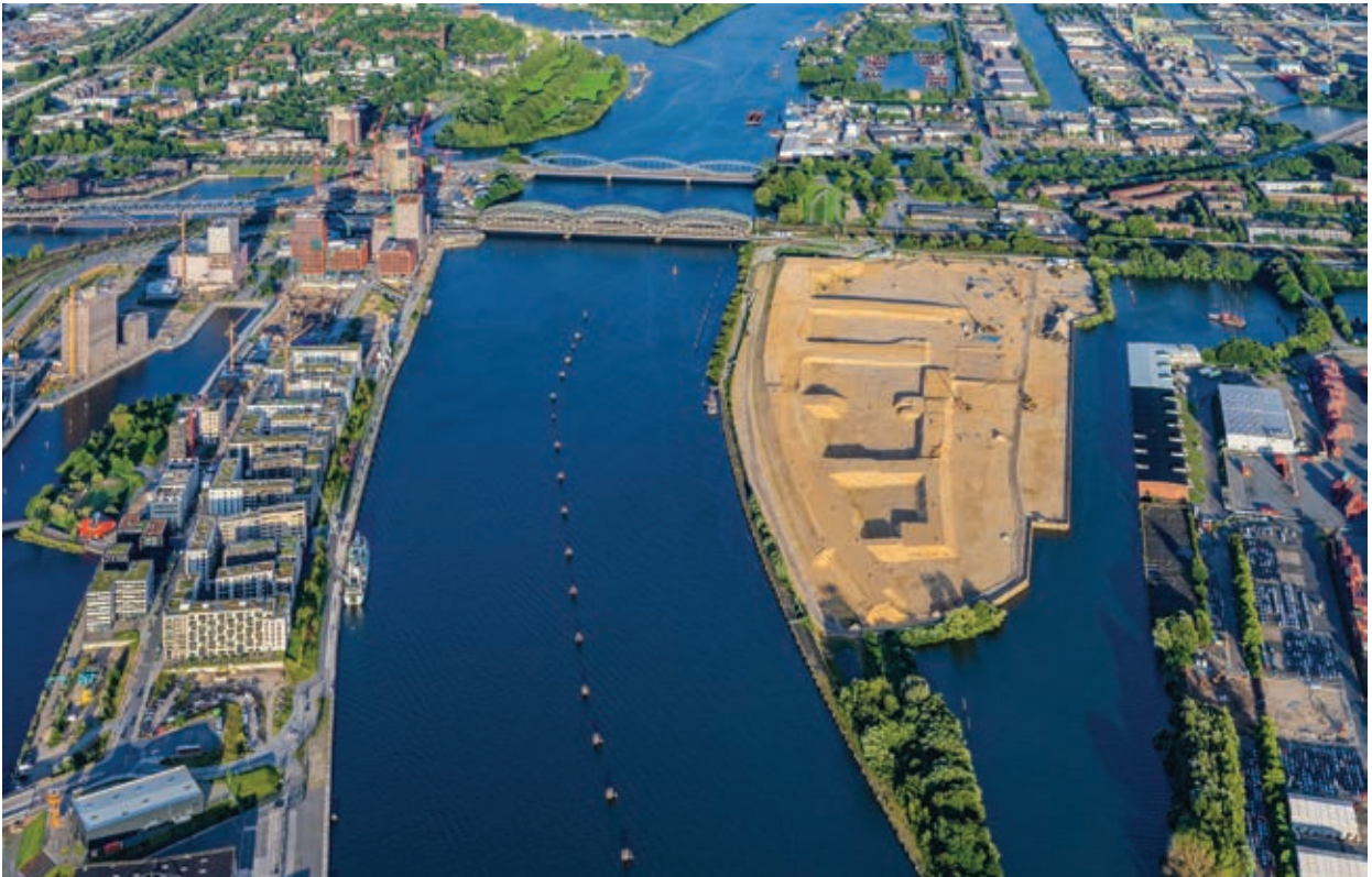
Kleiner Grasbrook (also known as the “Leap across the river” project). Preparation of the site is underway with terps (man-made mounds for flood protection) for buildings and streets. To its left is the final phase of HafenCity development. Image: Martin Elsen, Mediaserver Hamburg
